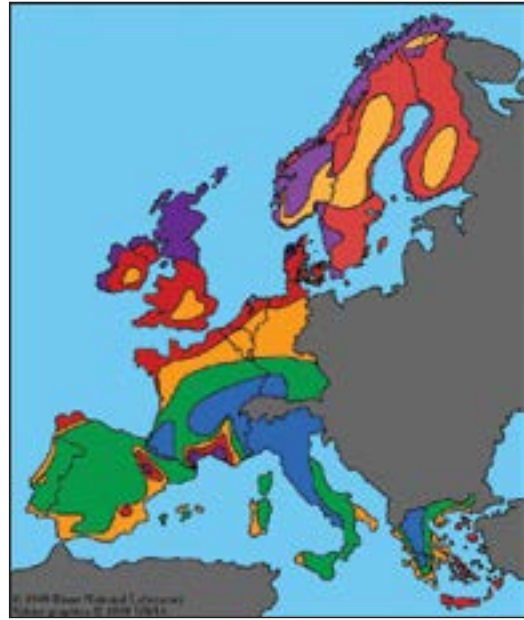
Figure 2.2-12: Wind speed (m/s) at 50 m above ground level for different topographic situations in Europe. (Troen and Petersen, 1989)
